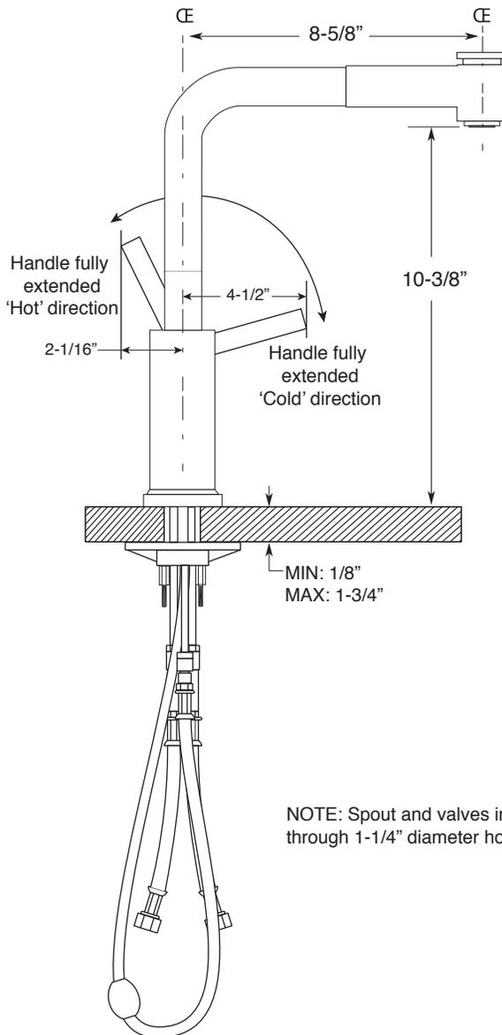
NOTE: Spout and valves install through 1-1/4" diameter holes
