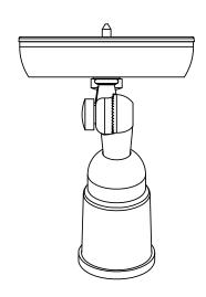
Suitable for wet locations when caulked to the mounting surface
