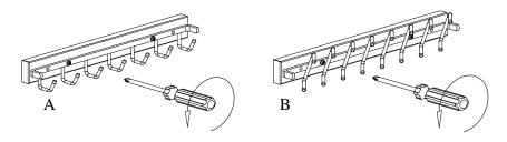
Step 2: Sliding out the housing and use 2 attached euro screws to fix slide on partition.
