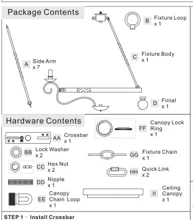
A. Attach the Crossbar (AA) to the Outlet Box with the head of the Green Ground Screw facing you. Secure it with Outlet Box Screws (not included). Tighten until snug.
