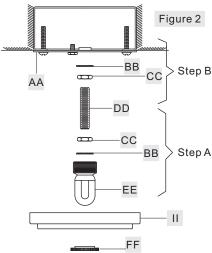
ceiling to determine the correct position of the Nipple (DD). Thread the Canopy Lock Ring onto the Canopy Chain Loop (EE). Adjust the Nipple (DD) to allow the Ceiling Canopy (II) to rest against the ceiling when held in place by the Canopy Lock Ring (FF).
