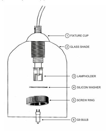
Note: Only operate with shatter resistant Sylvania CAPSYLITE® G9 bulb or equivalent.
