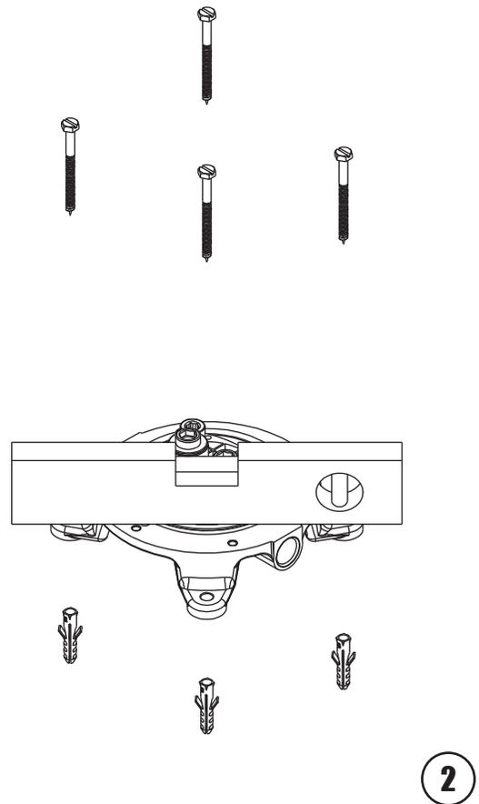
**2** Use the body as a template to mark the position of the screw holes in the subfloor. Fasten the body to the subfloor with the screws provided. Make sure that the body is level.
