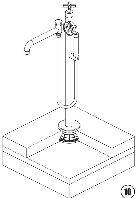
**10** To cover the protective cap, then to do water test and finish the installation.
