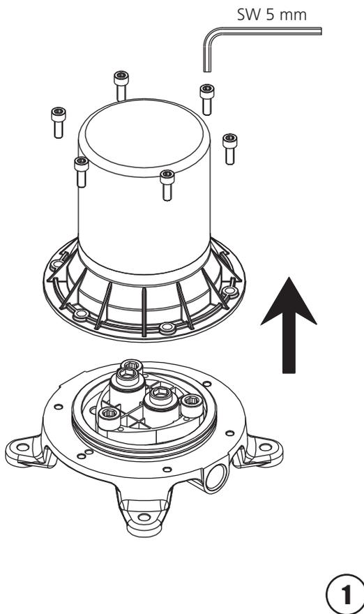
**1** Use a 5 mm Allen wrench to loosen the screws, then take off the protective cap.
