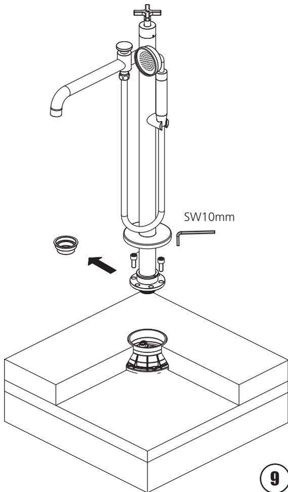
**9** Adjust the angle of the faucet and then install the faucet to the body with screws.
