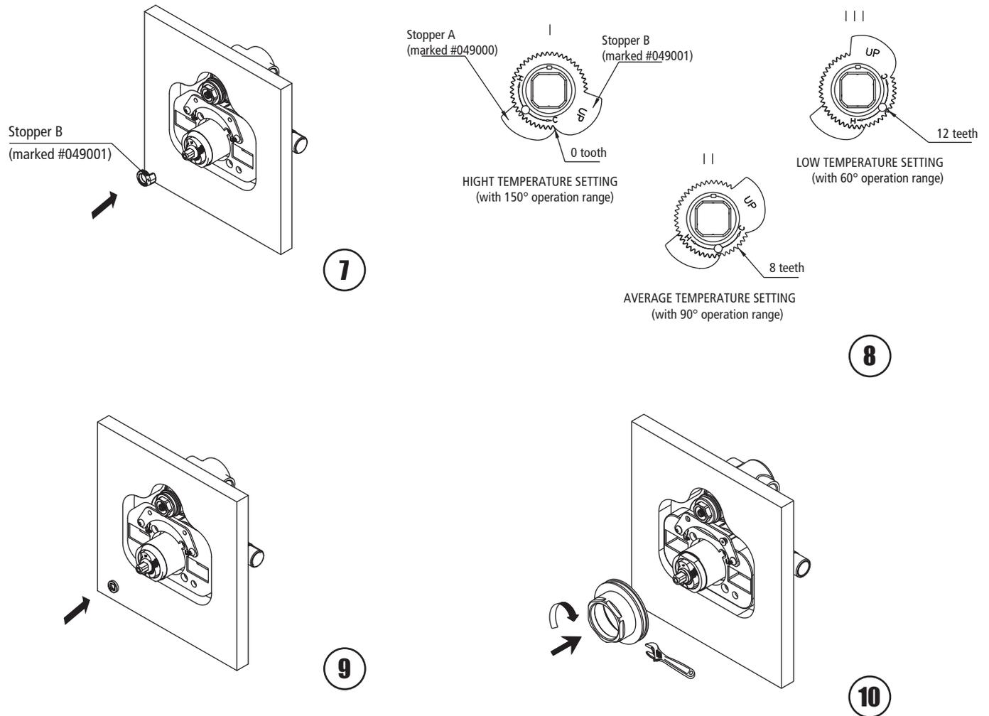
**7** Install stopper B. The word "up" should face out.
