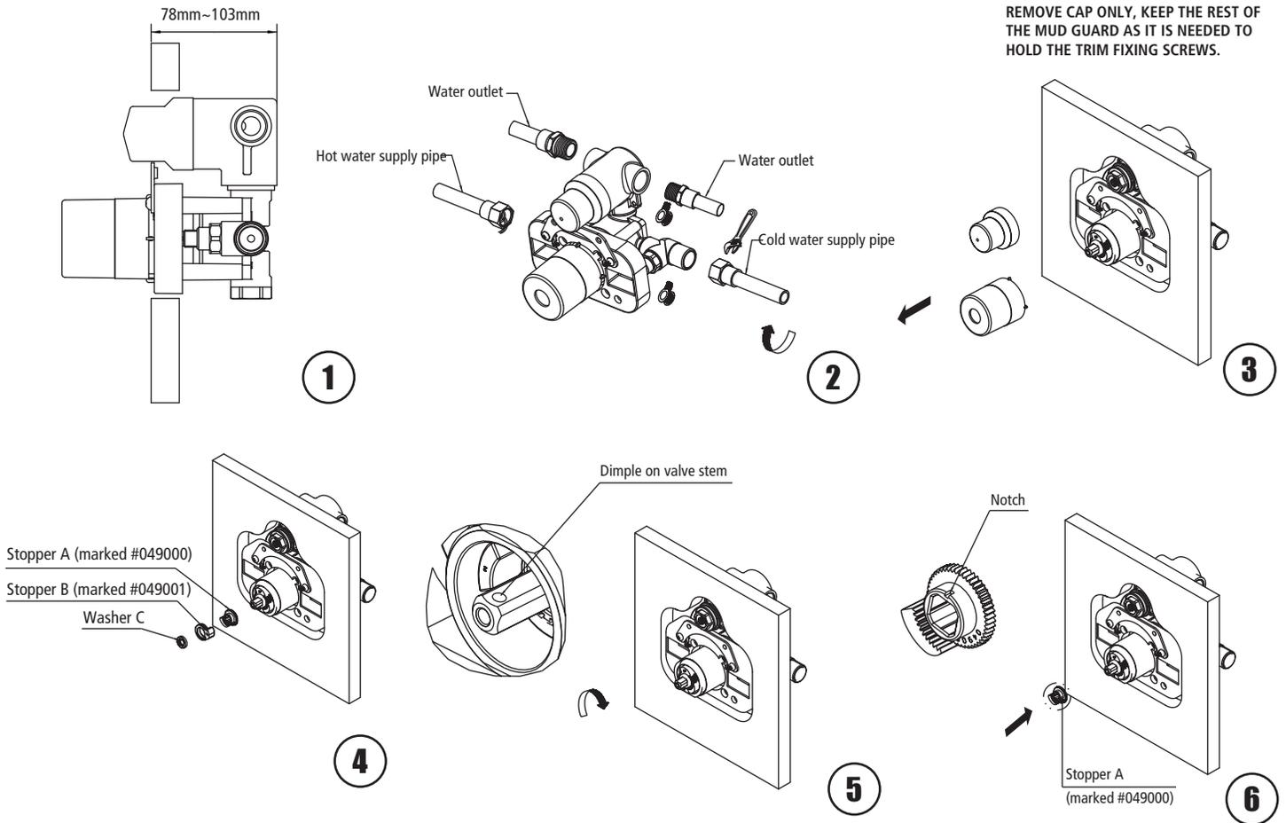
**1** While placing the valve into wall, make sure that the distance between the wall surface and the back of the valve is between 75~103mm as the figure indicates.
