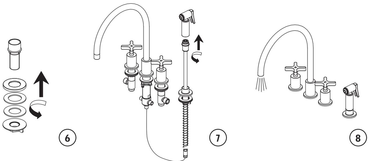
**6** Install spray holder in sink deck: insert the spray holder from above into the mounting hole. Tighten with lock nut.
