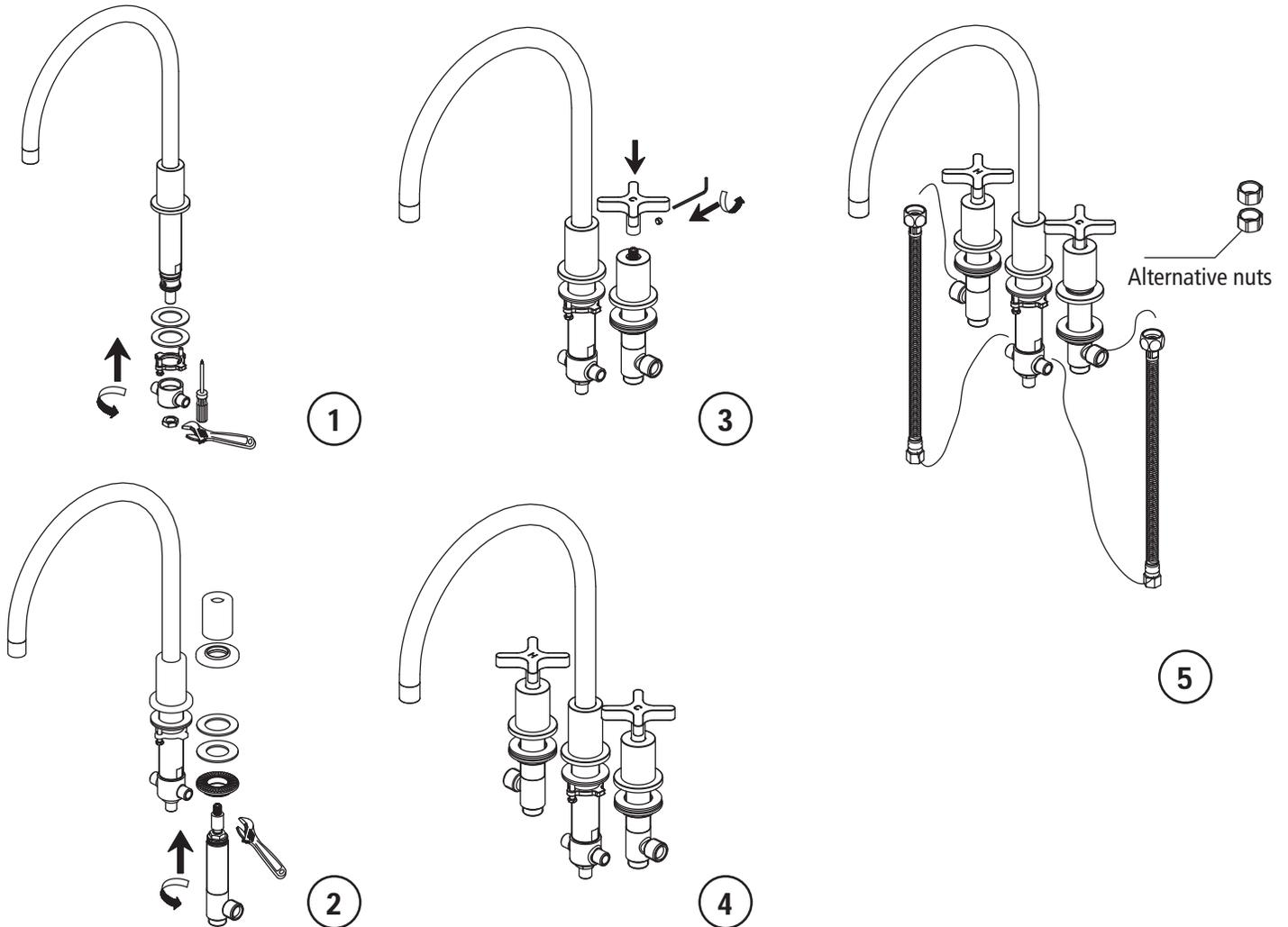
**1** Position the spout in the second hole of sink. Insert spout into the mounting hole in deck from above. From underneath the sink, install the washers and lock nut. Slide on adapter over bottom of spout shank, and tighten with lock nut.
