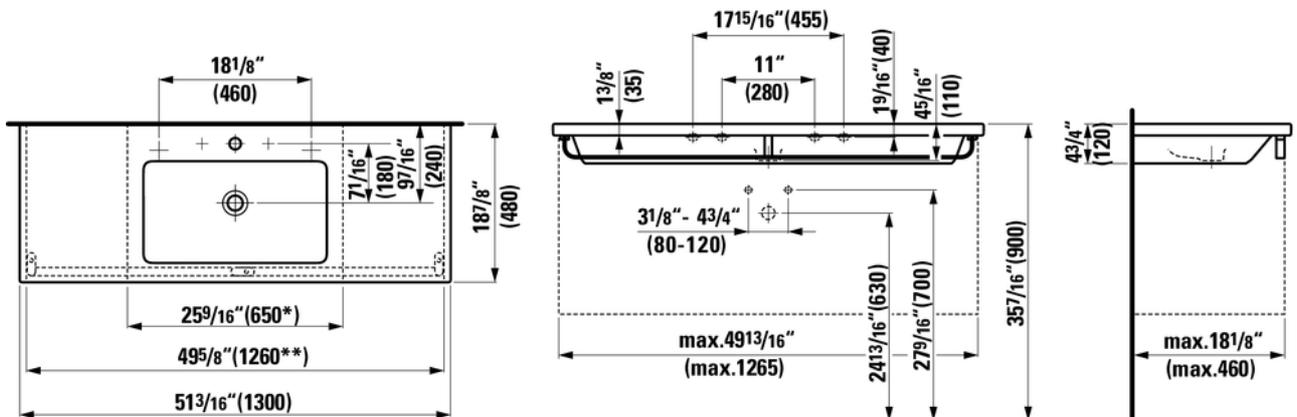
\* = minimum measure for cutting / \*\* = minimum measure for cutting with towel rail
