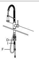
Connect the quick connector (I) to the supply hose (D) by twisting clockwise. Push the spray hose (F) firmly upward into quick connector. Pull down moderately to ensure the connection has been made.
