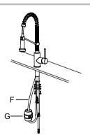
Install the weight (G) on the indicated mark on the spray hose (F).
