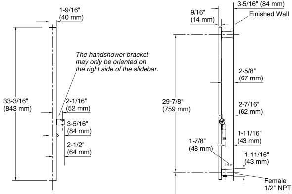
Recommended 48" (1219 mm) Floor to Bottom Post ADA Recommendation: 38" (965 mm) - 41" (1041 mm)
