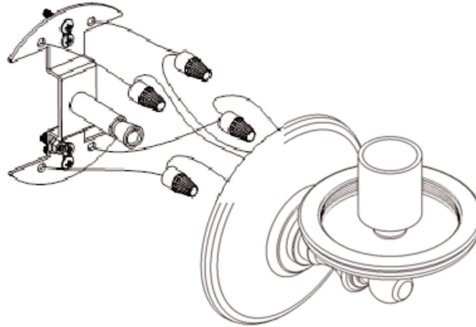
② MOUNT CROSSBAR TO ELECTRICAL BOX (NOT INCLUDED) USING #6 OR #8 SCREWS.
