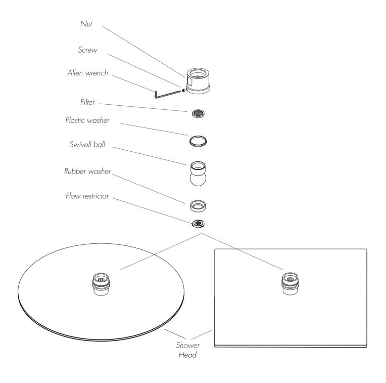
Auto Limited flow rate...... max 13 l/min
