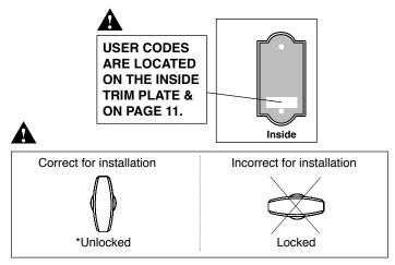
\*Unlocked position is required for installation and removal of the Inside Trim Plate Assembly.
