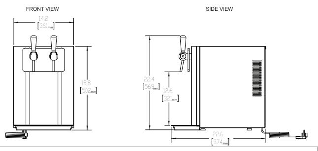
ELECTRICAL: 115 V -60 Hz. 1 Ph., 330 W – 3.2A, NEMA 5-15 Plug WATER SUPPLY: 3/8 in. supply recommended, 14.5 PSI min, 51 PSI max. (125 PSI max with use of supplied regulator) INSTALLATION: Provide 4 in. of clearance around unit to allow adequate ventilation **REQUIRES:** CO<sub>2</sub> tank with standard threaded connection to CGA 320 nut, **CO<sub>2</sub> TANK IS NOT INCLUDED**
