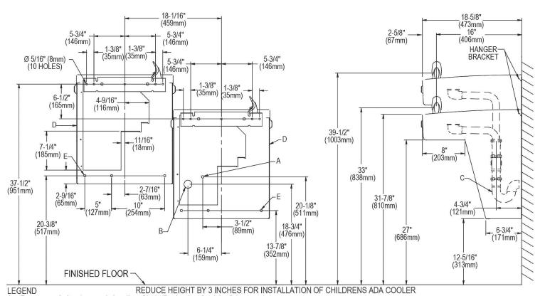
A = Recommended water supply location. Shut off valve (not furnished) to accept
