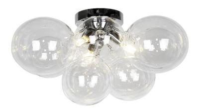
No. of Bulbs Height 11.625 Width/Length 14.188 **LED Compatible** Compatible Depth 14.188 **Total Wattage** 120W Weight 3.5 **Body Material** Metal **Second Material** Glass Finish/Color **Polished Chrome** Second Finish/Color Clear Type of Finish Electroplated **Bulb 1 Amount** 3 **Rated For** Damp **Bulb 1 Base Type** G9 Voltage 120V **Bulb 1 Max Watt.** 40W **Bulb 1 Included** No **Approval** cUL or equivalent **Bulb 1 Lumens** Warranty 1 Year **Bulb 1 CRI Instal Position** Ceiling
