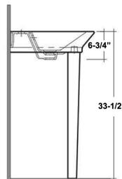
Dimensions of fixture are nominal and may vary within the range of tolerances established by ASME Standard A112.19.2.2018 Dimensions and specifications subject to change without notice.
