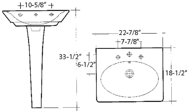
Dimensions of fixture are nominal and may vary within the range of tolerances established by ASME Standard A112.19.2-18. Dimensions and specifications subject to change without notice.
