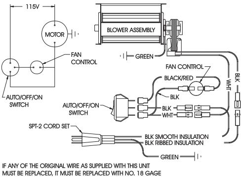
150°C 2/64 INSULATION WIRE OR ITS EQUIVALENT.
